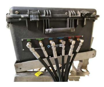
DIVING PANEL WITH D1/D2/D3 INLET (HP/LP) AND OUTLET FITTINGS (TO DIVER) FROM THE BACKSIDE OF THE **PANEL**
