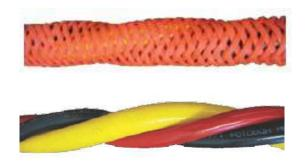
Lightweight, ultra flexible and kink resistant, Aquaflow Umbilicals are ideal for breathing gas supply, comms and pneumo service for surface demand umbilicals. They can be produced in production runs up to 740 meters long and can be over extruded or braided for additional protection against abrasion and use in contaminated waters.
